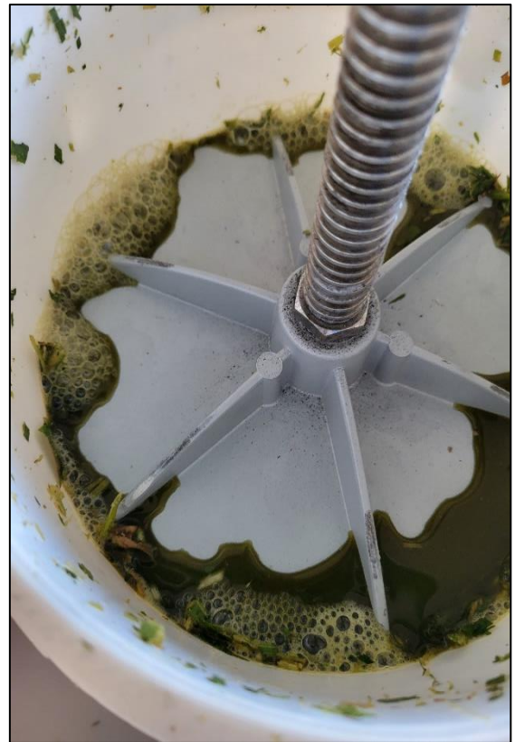
Figure 1. Leachate production from a male-sterile sorghum hybrid harvested with a 6 mm theoretical length of cut and 2 mm kernel processing roll gap with 77% moisture content after compression with a manual press.
